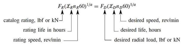
Solving for  $F_R$ , we obtain an expression for a catalog load rating as a function of the desired load, desired life, and catalog rating life.
