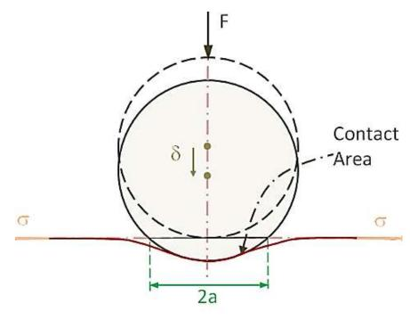
Elastic deformation yields a finite contact area.
