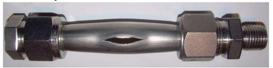
In some components yielding can also be considered as failure, if yielding distorts the material in such a way that it no longer functions
