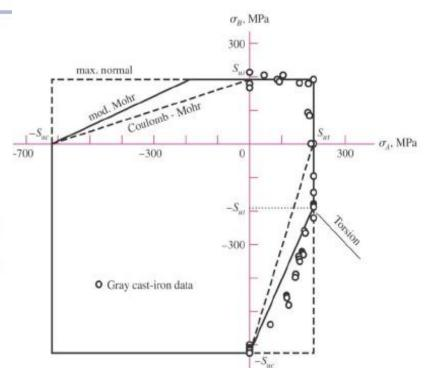
A cast pipe of outer diameter D = 100mm and inner diameter d = 60mm is made of an aluminum alloy having ultimate strengths in tension  $S_{ut} = 200$  MPa and compression  $S_{uc} = 600$  MPa. Determine the maximum torque that can be applied without causing rupture using maximum normal stress theory and a safety factor of n = 2. Reworked using Coulomb-Mohr and modified Mohr theories
