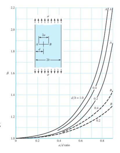
Given 2a = 65mm and found  $\beta \approx 1$ ; known  $K_{IC} = 28.3$ MPa $\sqrt{m}$ ; nominal uniaxial tensile stress  $\sigma = 50$ MPa and yield strength  $S_y = 240$ MPa
