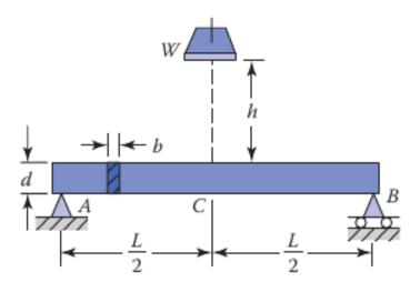
The maximum deflection, due to a static load, is  $\delta_{st} = \frac{WL^3}{48EI} = 0.154$ mm
