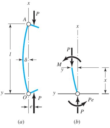
Note: maximum stress and deflection occur in the outermost fibers of the cross section at the mid-length of the column
