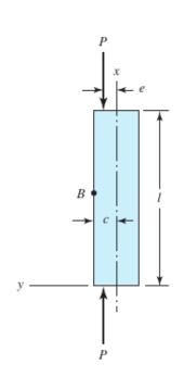
A piece of work in the process of manufacture is attached to a cutting machine table by a bolt tightened to a tension of T. The clamp contact is offset from a centroidal axis of the strut AB by a distance "e" as shown. The strut is made of a structural ASTM 36 steel of diameter d and length L. Given: The numerical values are d = 30 mm, e = 3.5 mm, L = 125 mm, T = 2P = 7 kN, E = 200 GPa, Find the largest stress in the strut. Assume strut is pinned at both ends.
