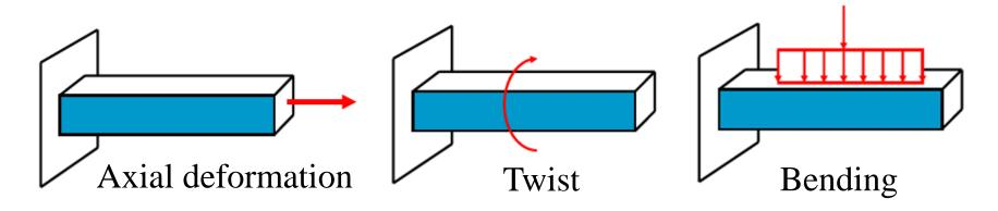
Axial loading (tension +ve/compression -ve)
