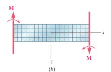
Normal stress and shearing stress due to bending
