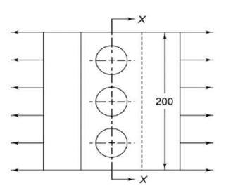
Given P = 50kN, (fs) = 2.5,  $S_{vt} = 250 \text{ N/mm}^2$ ;
